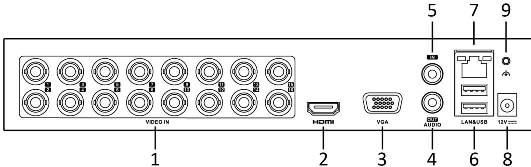
\*: The rear panel of DS-7204/7208HQHI-K1/E provides 4/8 video input interfaces.
